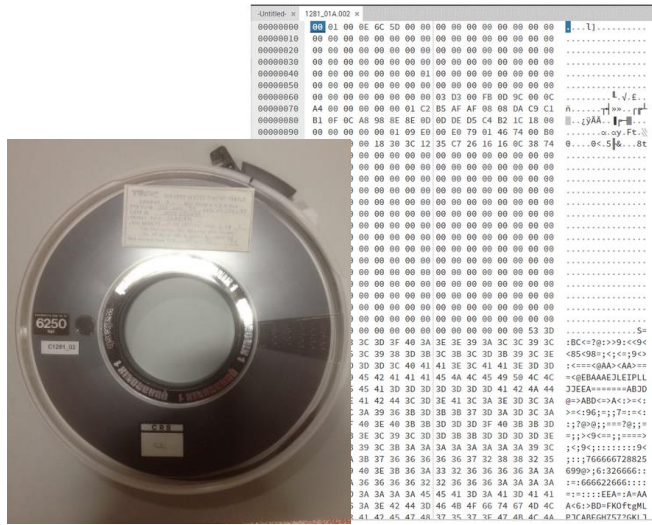
Fig. 2. One of the 9-Track 1/2" Magnetic Tape which stored the original Landsat data. The bit sequence from one of the Landsat files rendered via a hex editor in 2020. Quelle: Doig (2020) https://www.dpconline.org/blog/james-doig-preserving-the-bits
